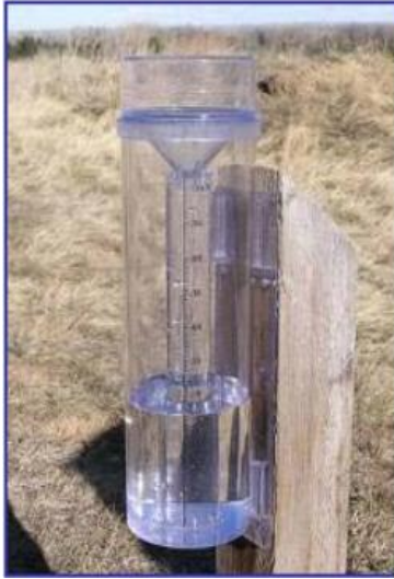
Manual rain gauge from the Community Collaborative Rain, Hail & Snow Network (CoCoRaHS).
