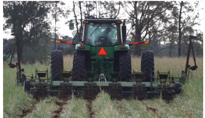
Figure 2. Custom roller/strip-till implement by Myron Johnson of Headland, Alabama. Credits: Brian Kahn.
