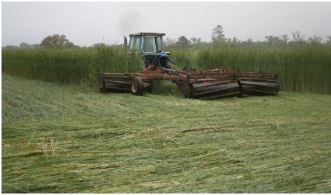
Figure 1. Cereal rye cover crop rolling/crimping in late March 2011 at Brock Farm in Monticello, Florida. Custom roller/crimper design and fabrication by Kirk Brock. Credits: Danielle Treadwell.
