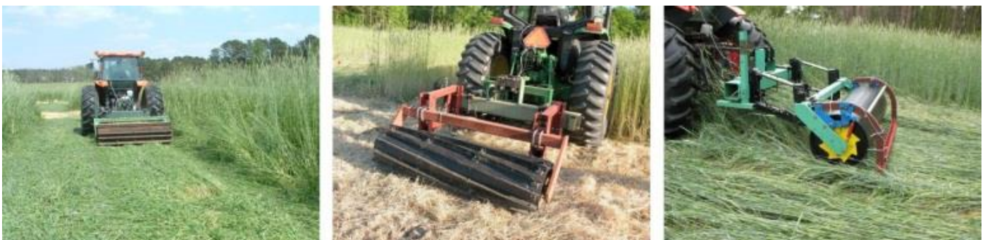
Figure 3. From left to right: straight-bar, curved-bar, and smooth/crimper-bar roller designs. Credits: Ted Kornecki, USDA-ARS.
