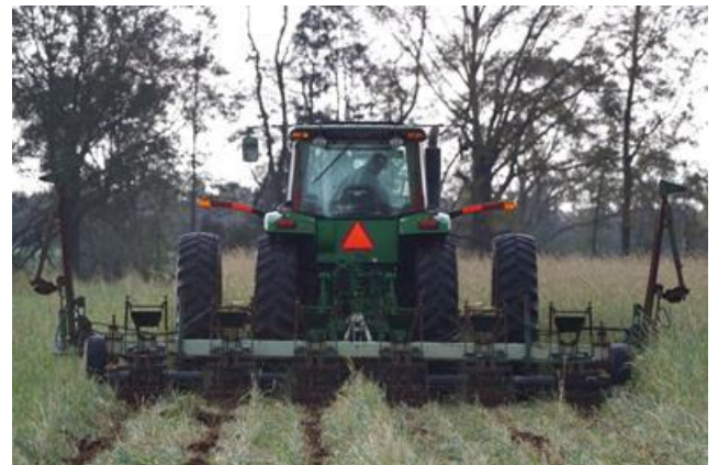
Figure 3. Cover crop rolling and strip tillage in preparation for planting; note the substantial plant residues maintained on the soil surface. Custom roller/strip-till unit by Myron Johnson of Headland, AL. Credit: Brian Kahn.
